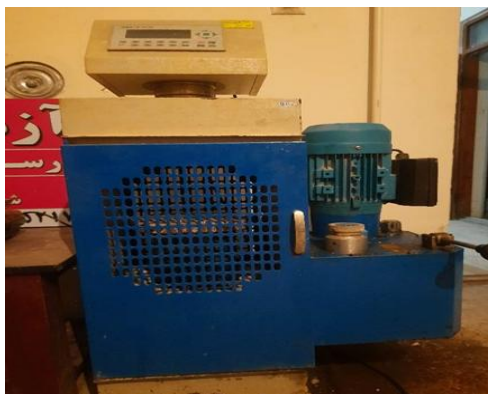
Fig. 5. Concrete compressive strength determination device.
