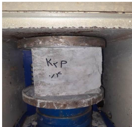
Fig. 11. 28-day concrete sample with 0.4% fibers.
