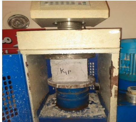
Fig. 9. 28-day sample with 0.2% rock wool fibers.
