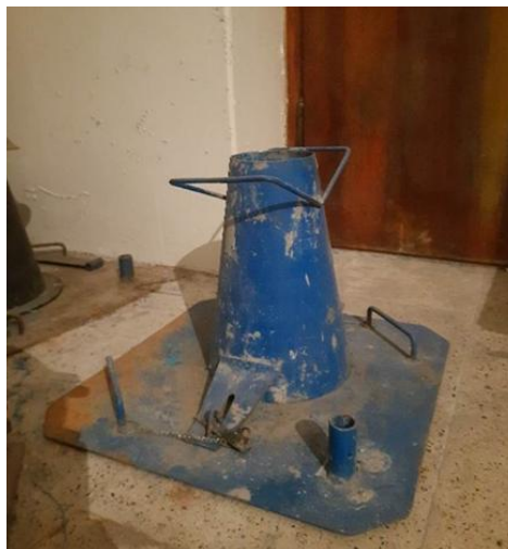
Fig. 6. Slump test mold.
