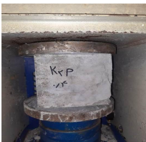
Fig. 11. 28-day concrete sample with 0.4% fibers.
