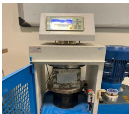
Fig. 3. the concrete breaker jack for the test to determine the compressive strength.
