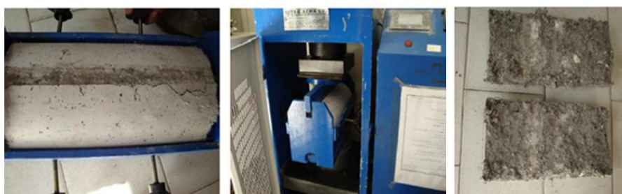
Fig. 5. Testing to determine the tensile strength of cylindrical specimens using the Brazilian method.
