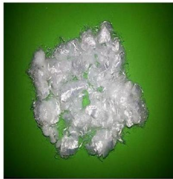
Fig. 1. Polypropylene fibers after separation by hand.
