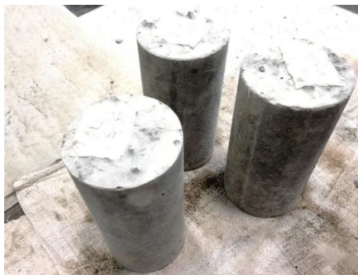
Fig. 4. Cylindrical samples for testing tensile strength.
