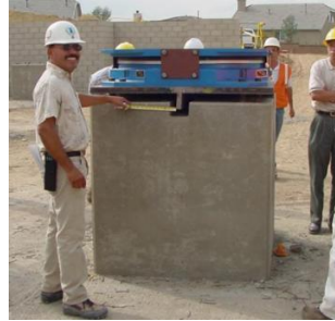
Fig. 3. Friction pendulum seismic isolator system (FPS).
