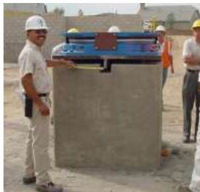
Fig. 3. Friction pendulum seismic isolator system (FPS).
