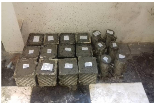
Fig. 8. A view of concrete poured in standard molds.
