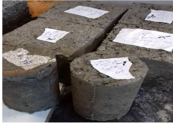
Fig. 9. Concrete samples after removing from the molds.
