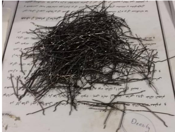
Fig. 3. Metal fibers with two hook ends with a diameter of 0.5 mm.
