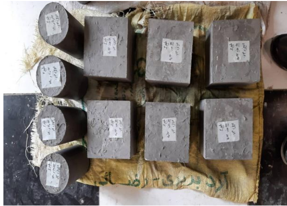
Fig. 7. Concrete samples after being removed from the mold.
