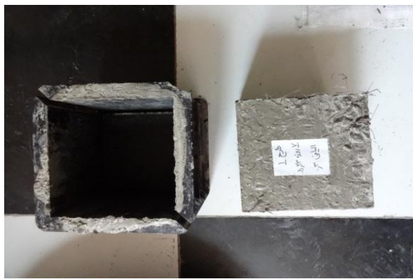
Fig. 8. Concrete samples 24 hours after construction.
