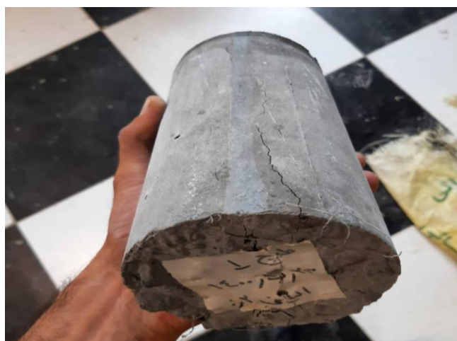
Fig. 13. Cracking pattern of concrete samples after tensile test.
