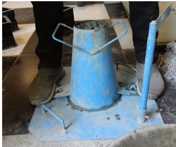
Fig. 9. Poured concrete in the slump cone.
